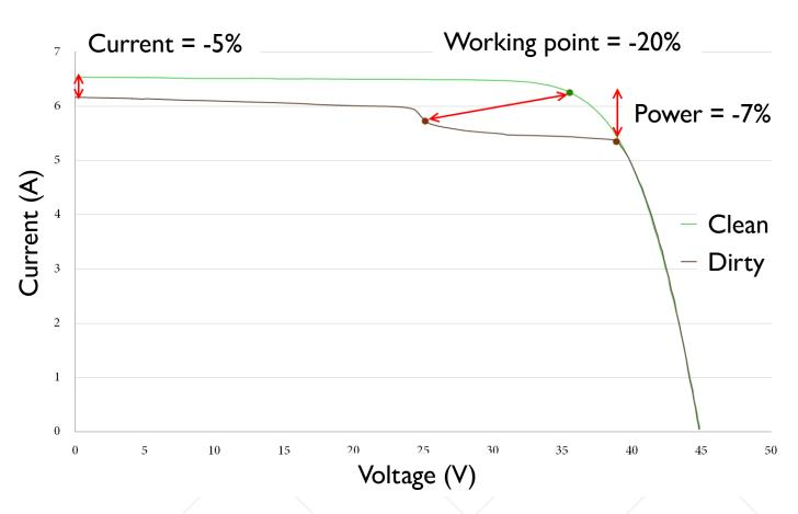
Key approach: PV modules as sensor + measure the effective impact
