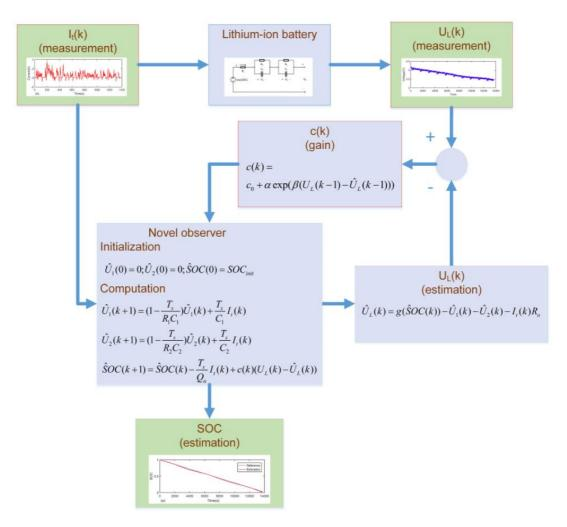
As the battery cell ages, the estimation error increases due to the variation of model parameters. To keep the accuracy of SOC estimation under acceptable limits, it is possible to update the parameters through a SOH estimation. In [163], for offline parameters recalibration and SOH estimation, a fourth order EKF is used.
