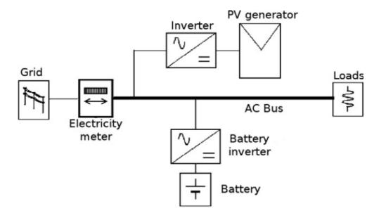
Figure 3.2: Topology of the power system in a building with BIPV, storage, consumption and grid connection. Source [111].
