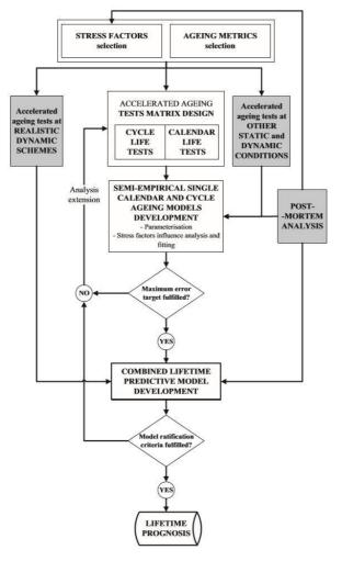
Figure 4.10: Flowchart of methodology for lifetime prognosis by [160]
