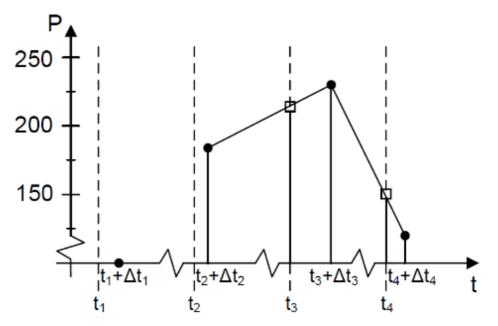
Figure 2.1: Example of asynchronous power measurement corrected by linear interpolation. Source [16].
