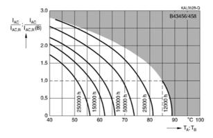
Figure 4.2: EPCOS/TDK capacitor lifetime as a function of temperature and current ripple.
