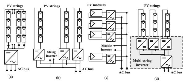
Figure 3.1: Configurations of grid-connected PV inverter [59]
