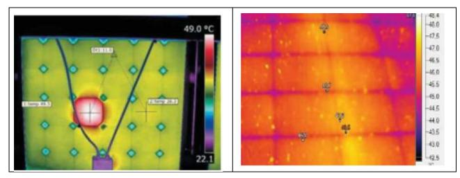
Figure 6.1: Images obtained from an IR inspection for cells anomalies and hotspots identification respectively
