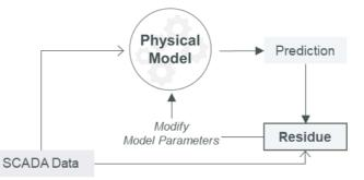
Figure 4.1: Optimization of a physical model to transform it into a hybrid model.
