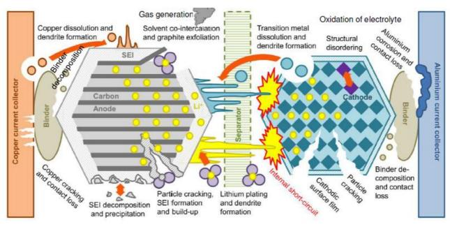
Figure 4.8: Degradation mechanisms in a battery [168]
