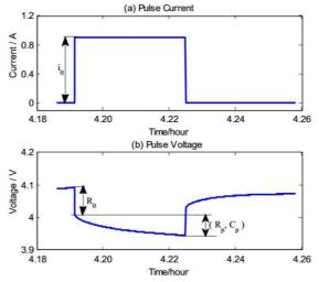
Figure 4.7: Zoom into discharge pulse of the LiNMC cell at around 90% SOC at 22°C [163]
